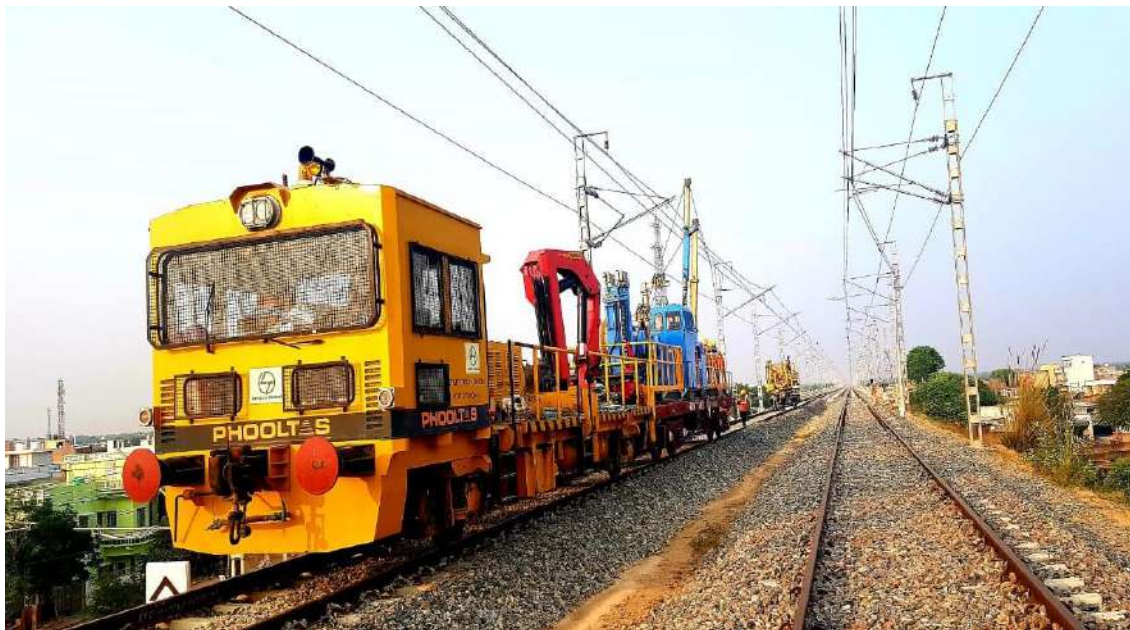
Mechanized wiring train for simultaneous wiring of OHE conductors
