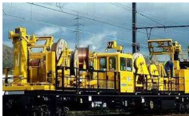
Simultaneous stringing of Contact and Catenary Wire by self-propelled wiring train
