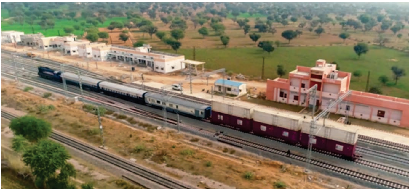
Successful Oscillation trials for 25 tn axle load trains at 110 kmph in Rewari-Phulera section of WDFC on 20.01.2020
