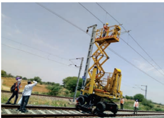
Mechanized inspection of works using rail borne vehicles such as Vertical Cradle Platform (VCP) and tower wagon etc.
