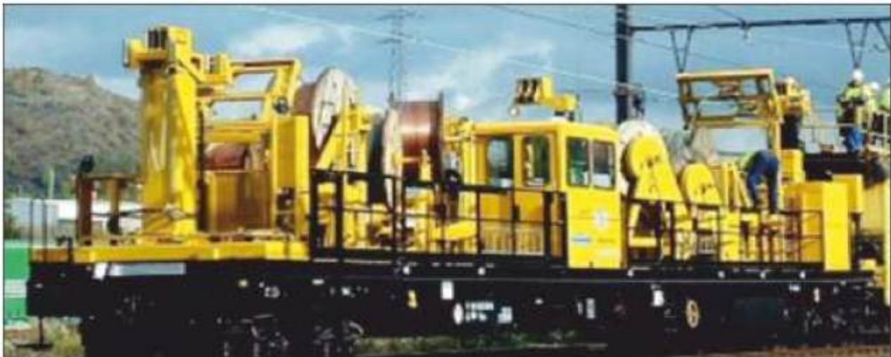
(Simultaneous stringing of Contact and Catenary Wire by self propelled wiring train)
