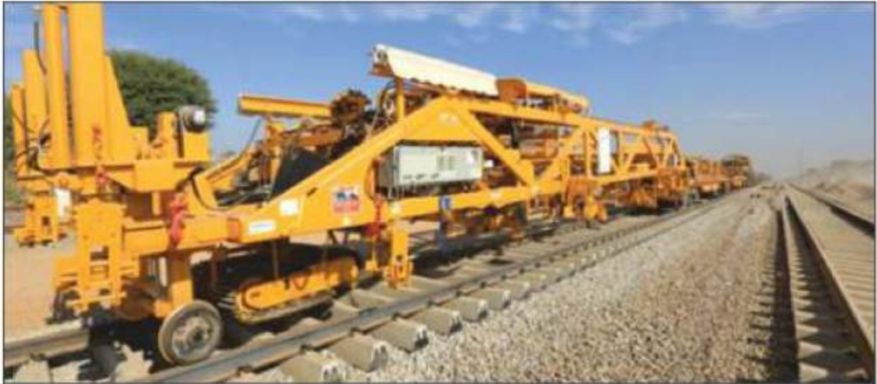
Advantages of track linking by NTC machine as compared to conventional track linking:
