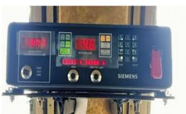
Acoustic Bearing Detector (ABD): ABD is a technology engineered to enhance safety & efficiency of Rail Transport. Roller Bearing's health is one of the decision makers in deciding the safety of Rail Transport. Trackside Acoustic Detection System is designed to monitor roller bearings and identify the same with internal defects prior to overheating, costly train stops, and ultimately failure. This technology enhances equipment performance and prolongs infrastructure life.
