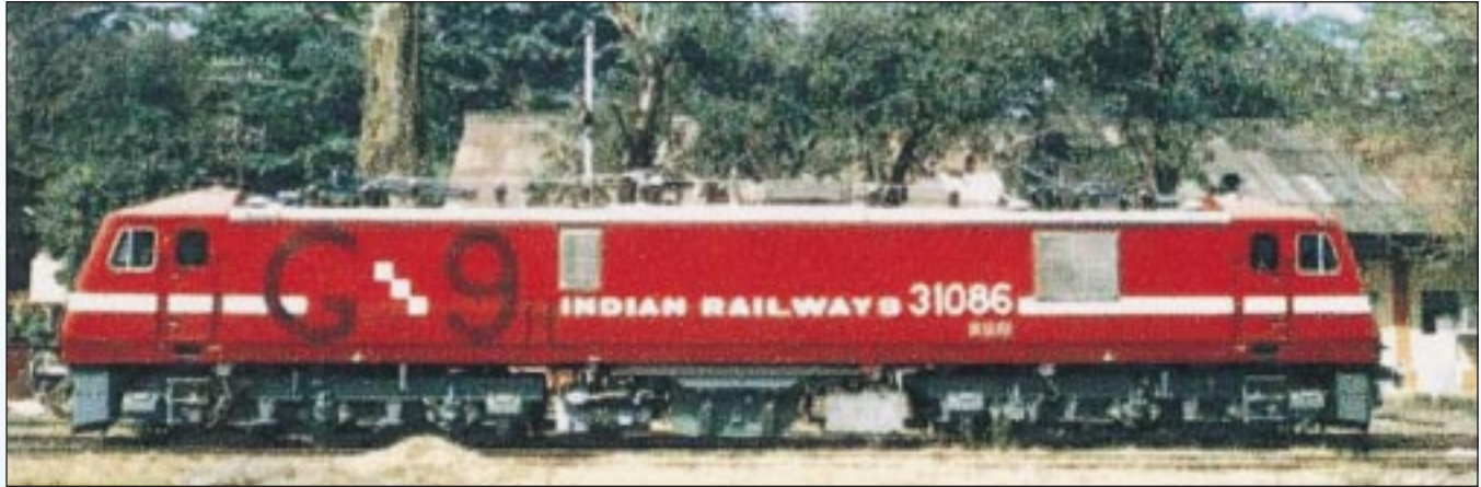
Dr. Silver : WAG-9H- phase Electric Engine with remote diagnostic System.
