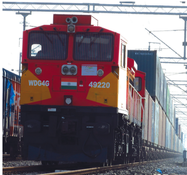
Three Phase Electric Locomotive with Regenerative Features
