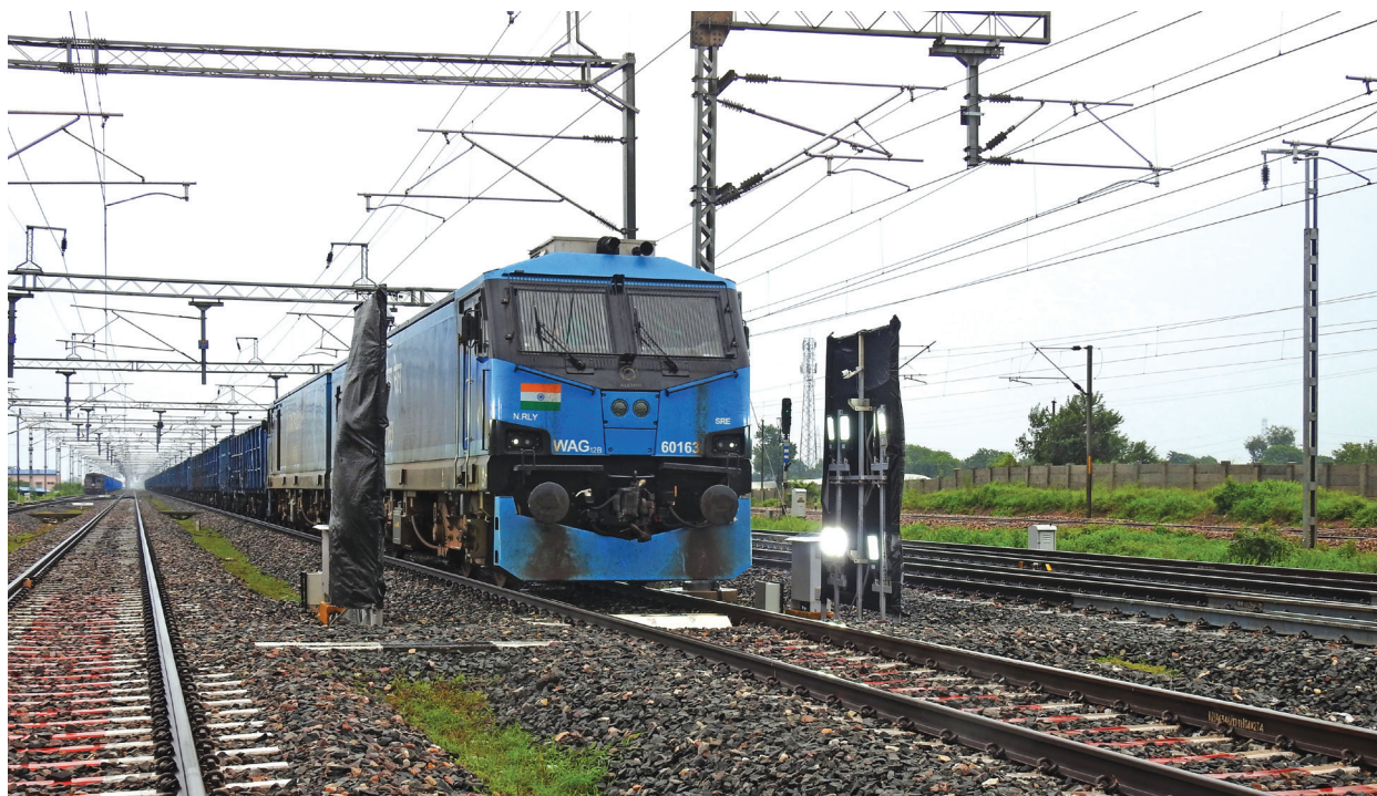
MVIS System Installed at New Daudkhan Station of EDFC
