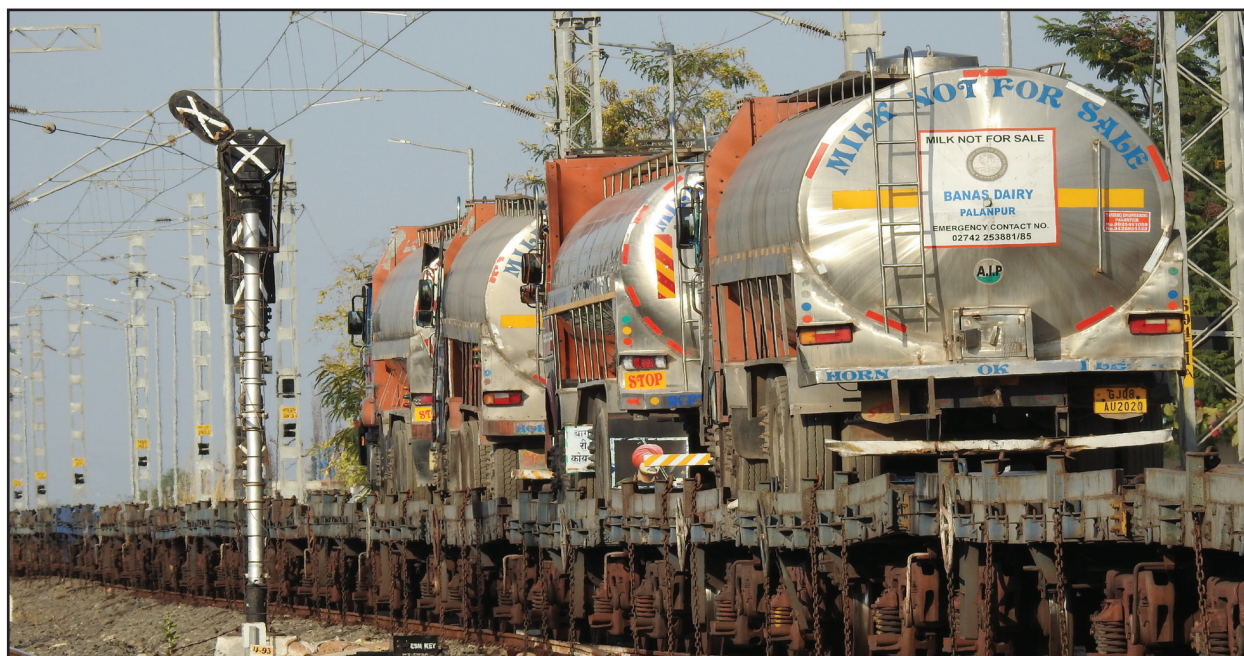
Truck-on-Train service carrying milk tankers on the New Palanpur-New Rewari stretch.
