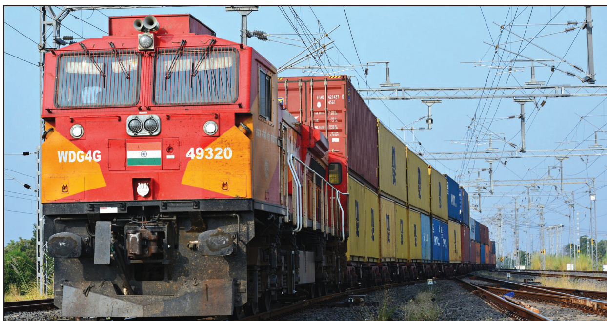
WDG-4G locomotive hauling double stack container train near Palanpur.
