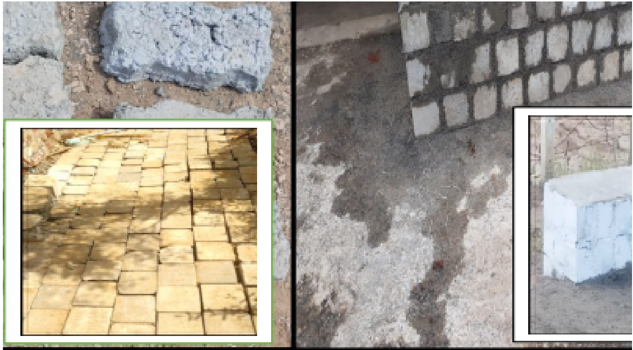
Fig 3: Concrete waste being used to make bricks for further use
