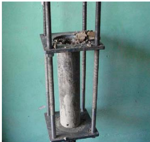
SAMPLE EXTRUDER (SOIL) HYDRAULICALLY OPERATED
