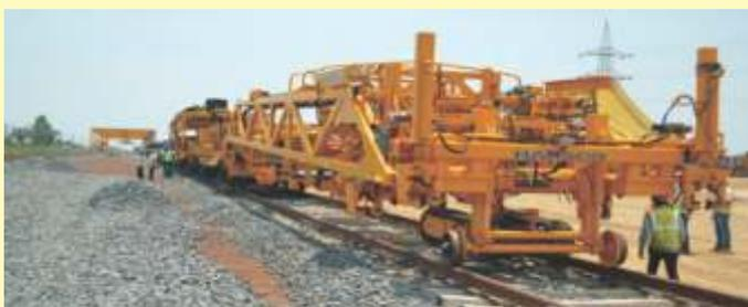
Mechanised Track laying by NTC Machine
