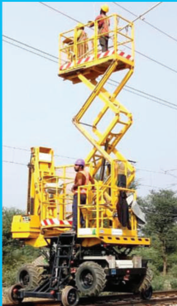
Fig. 11: RRV mounted vertical cradle platform
