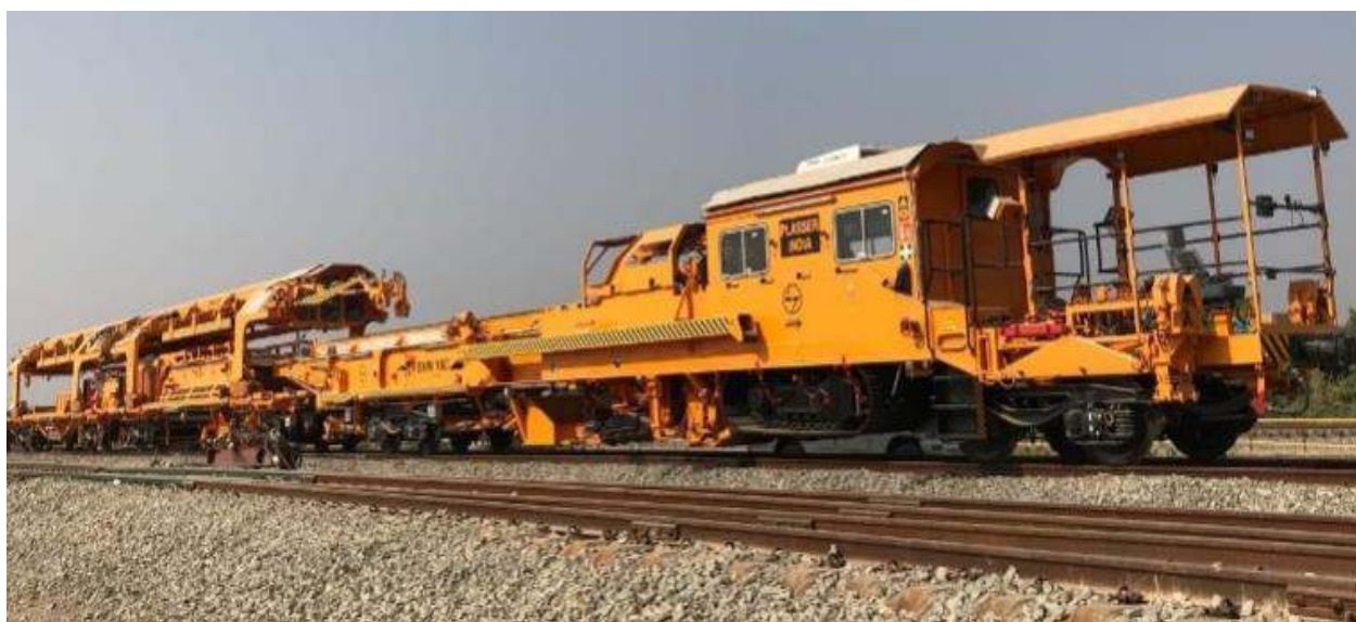
Fig. 6: NTC track laying machine
