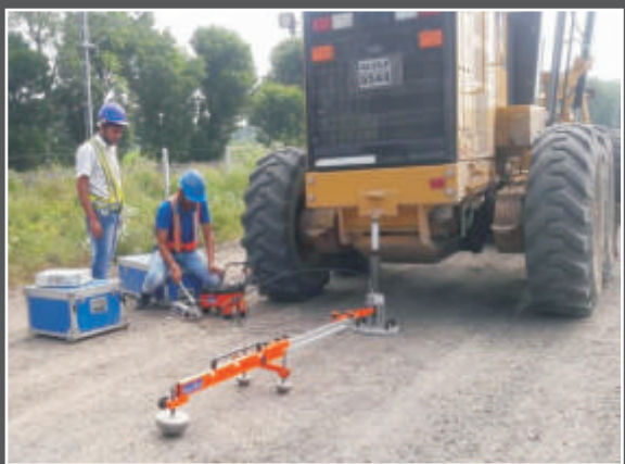
Fig. 3: Field EV 2 load test measurement
