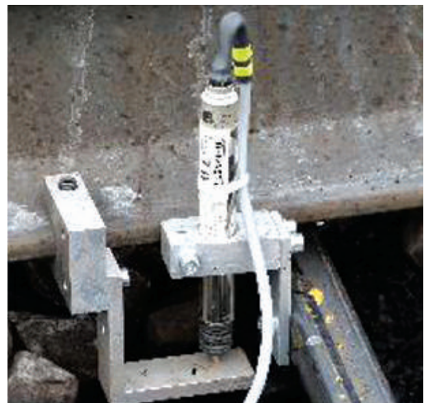
Figure 3: Deflection measurements at the transition zone (top). Determining the contact area in the lab (bottom).
