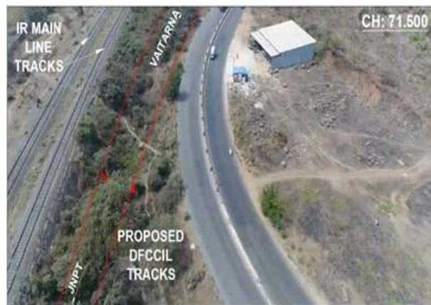
Figure 8. Diversion of state highway for tracks
