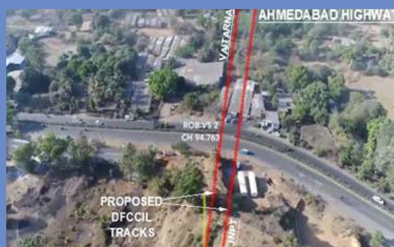
Fig.1b Alignment crossing highway and PAPs
