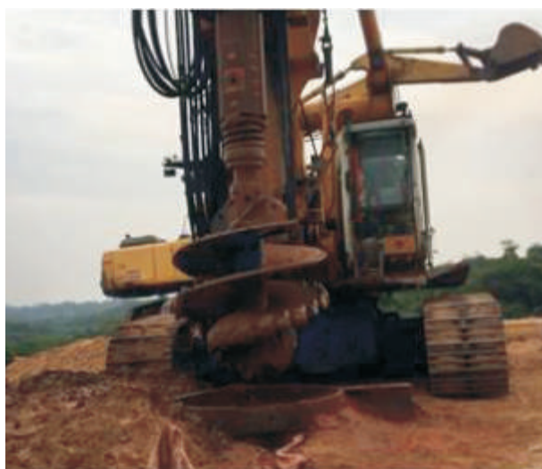
Fig. 4: Hydraulic rotary pile drilling rig
