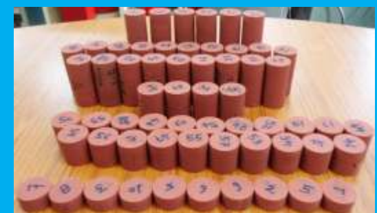
Figure-8 Preparation of Rock Specimen for Testing
