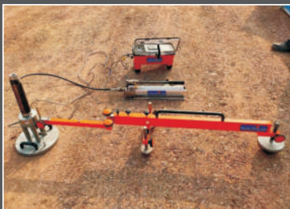
Fig. 2: EV 2 plate load test equipment
