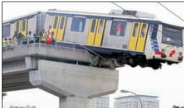
Figure -1: Overshooting of train due to inadequate Buffer stop
