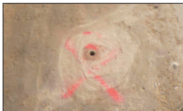
Figure 11: The site for the NDG must be flat and the hole prepared such that it is circular
