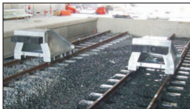
Figure-3: Sliding 'friction' end stop – non-hydraulic
