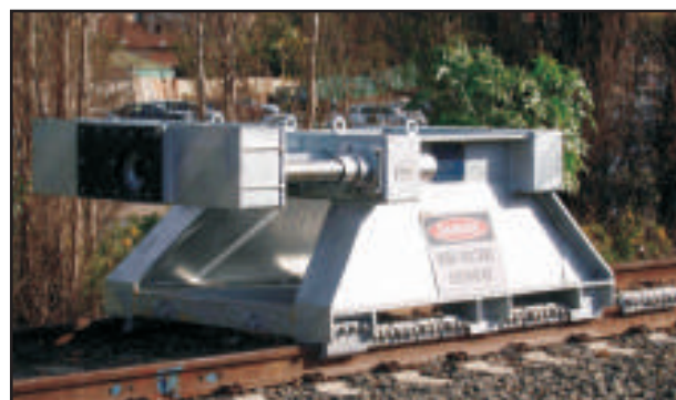
Figure-2: sliding friction end stop
