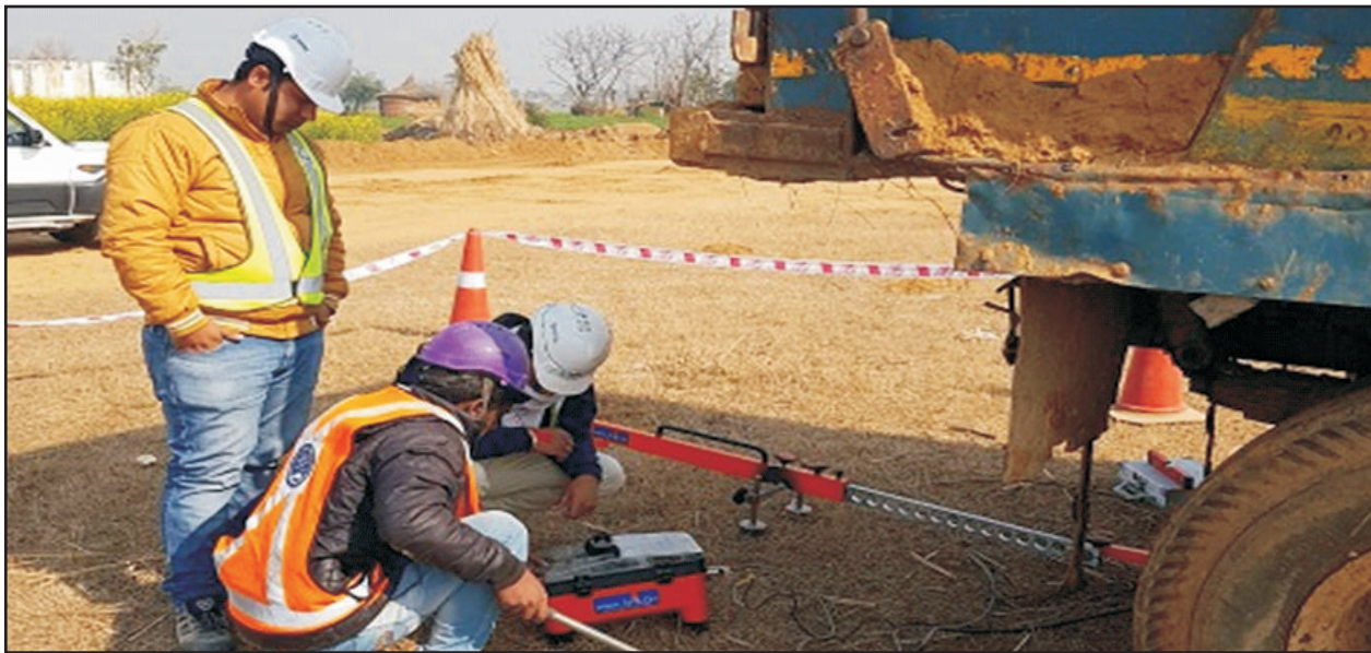
Fig 4 : Second Step Plat Load Test (Ev2) Conducted on Sub Soil
