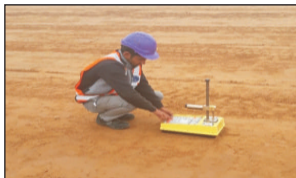
Figure 12 : Checking of compaction of soil by using Nuclear Density Gauge
