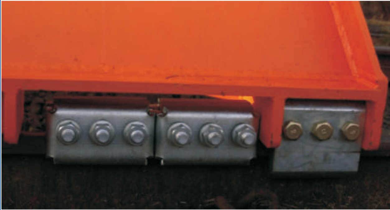
Figure -6: Friction Buffer Shoe with anti climb Stopper
