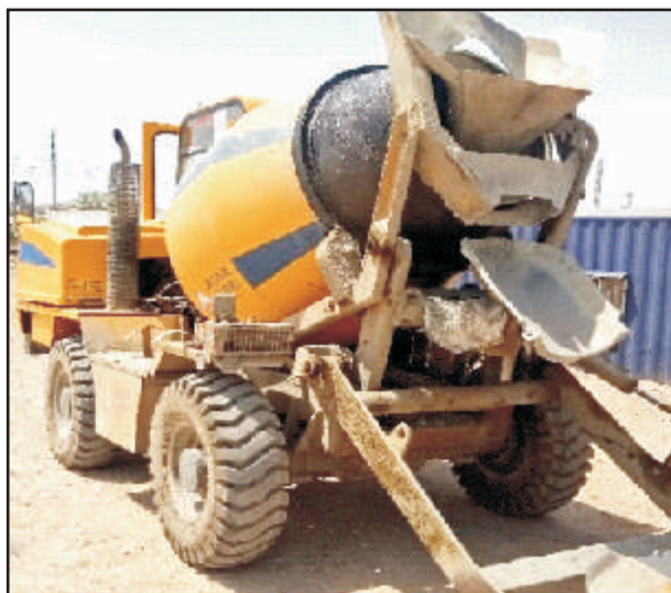
Fig.-5 Concrete self loading mixture
