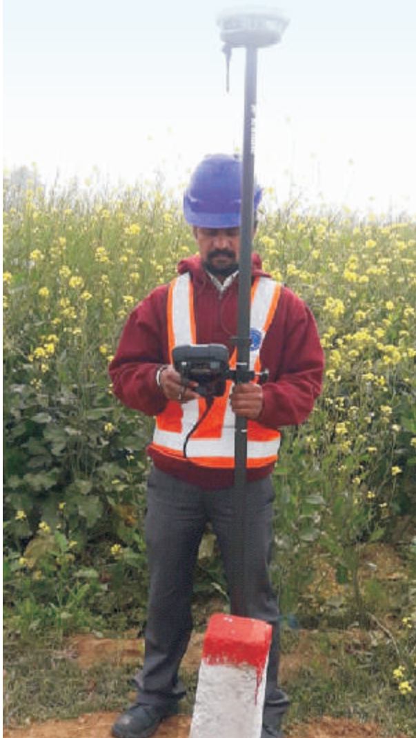
Fig-11: DGPS observation in RTK mode for ROW validation
