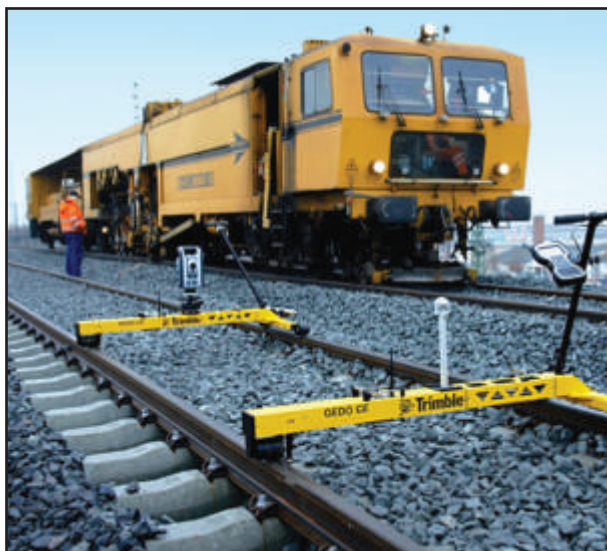
Fig -Trolleys- One with robotic total station and other with prism and controller unit
