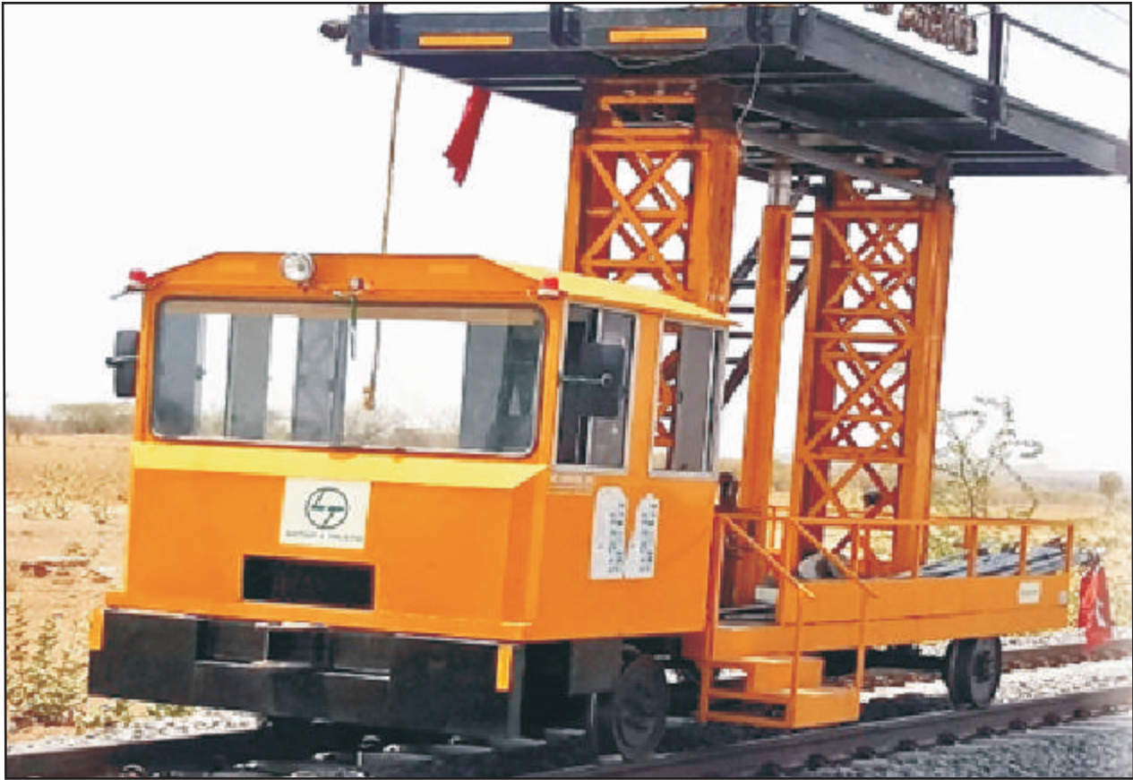
Fig.-15 Rail based cantilever adjustment vehicle
