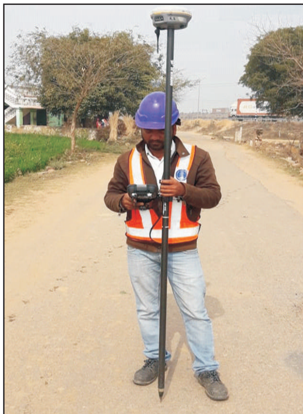
Fig.-12 DGPS observation in RTK mode for Topographic Survey
