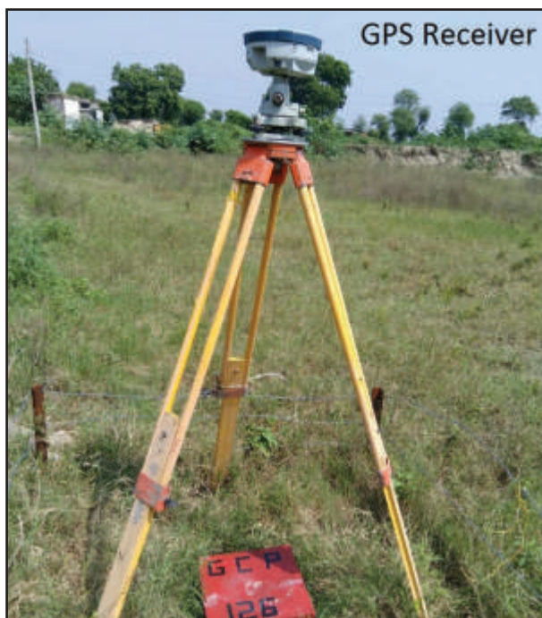
Fig.-7 DGPS observation in Static mode at 5Kms. interval Bench Mark Pillars
