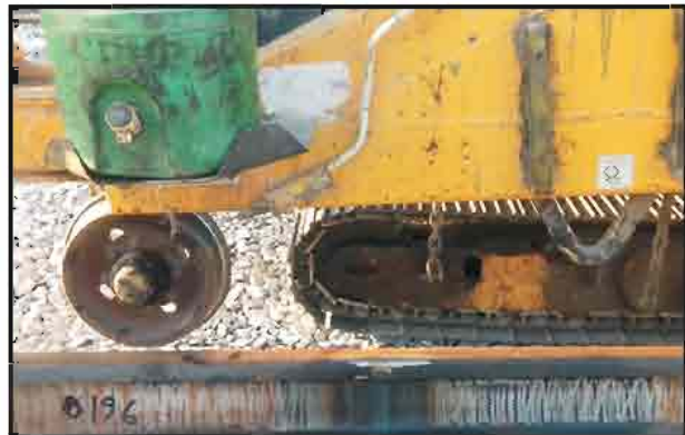
(c) Crawler on which truss frame is supported in front and moves on ballast bed during working.
