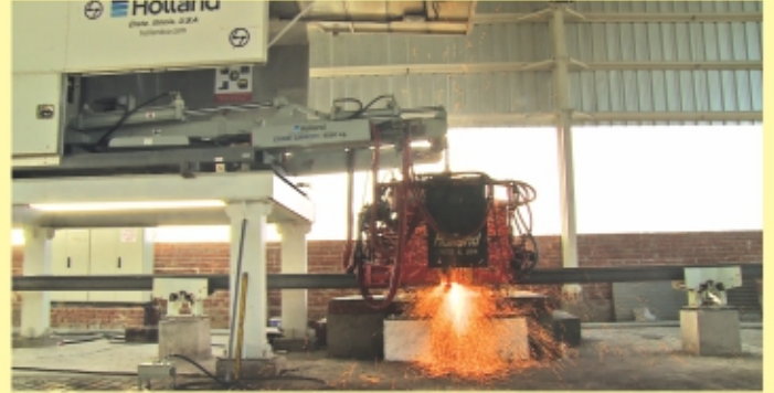
WDFC- Welding by Flash Butt welding plant in progress
