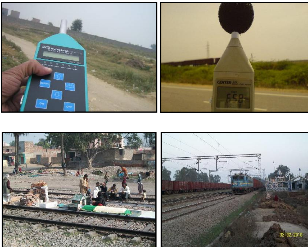
Fig. 5.12: Ambient noise monitoring
