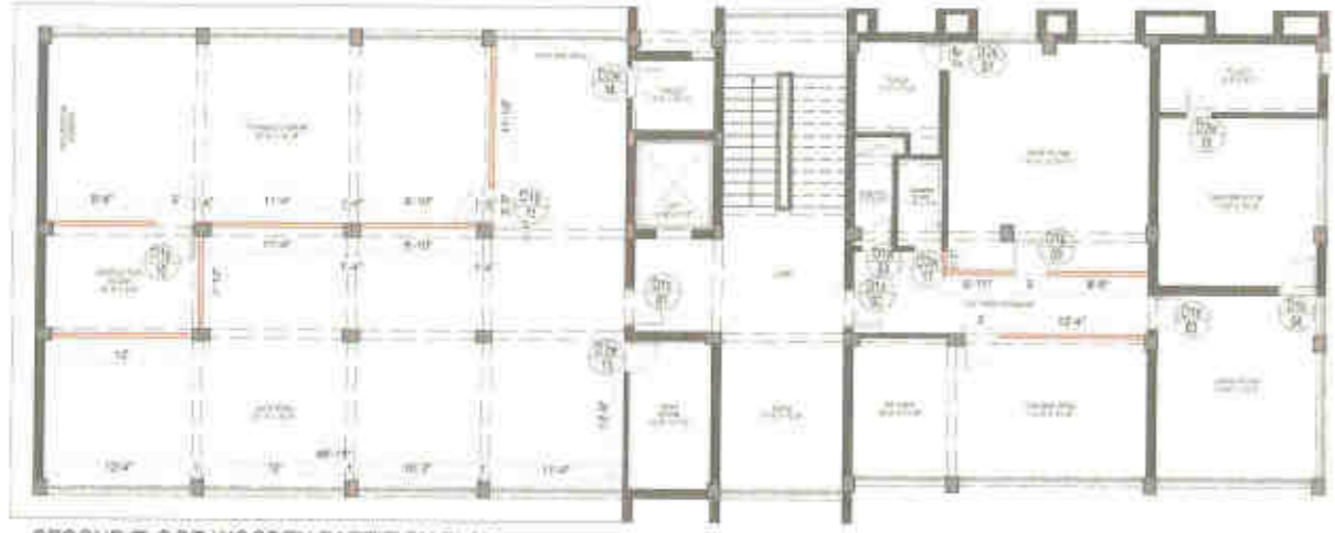
SECOND FLOOR WOODEN PARTITION PLAN
