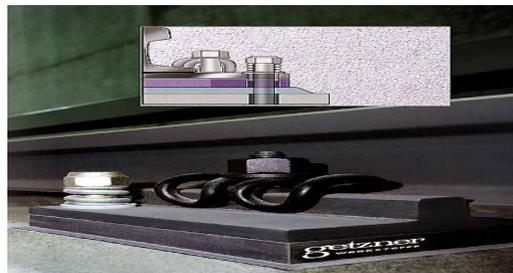
Special fasteners with vertical dynamic stiffness in the range of 8 kN/mm will reduce vibration by as much as 15 dB at frequencies above 30 Hz. (Conservatively these could **reduce vibrations by 5 to 10 dBs**). **Fig- 8.1** shows a typical resilient fastener.
