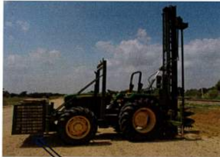
Counter weight mounted in the tractor
