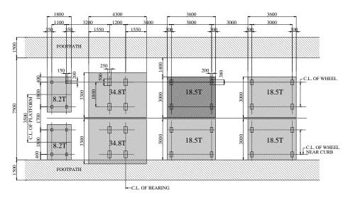
PLACEMENT OF 2-LANES OF IRC CLASS-A LOADING AND FOOT6PATH LOADING ON CARRIAGEWAY
