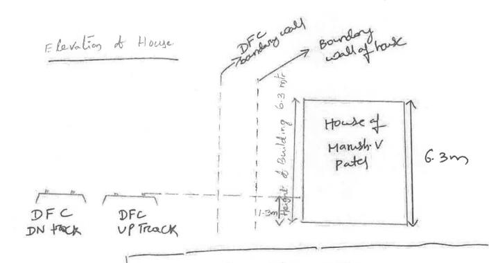
Height of boulding = 6.3m Height of boulding from top of DFC Uplane Height from ground level = 63m = H clearance required = 1/2 = 3.15 m EXE GONDEL Clearance from Railway boundary = 7.55m = 07 04.2025 Gad avil /AL 07:04.2025
