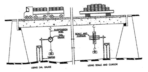
The deflection measurement can be done by suspension wire method at the required locations using dial gauges (Fig.). In this method trestles or posts 1.5m tall would be embedded in firm ground and dial gauges of least count 0.01 mm are clamped to them. The spindles of the dial
