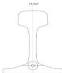
Fig.4(a) The location of sample for YS, UTS and Elongation in rail foot for R260 grade rails
