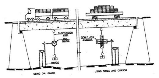
The deflection measurement can be done by suspension wire method at the required locations using dial gauges (Fig.). In this method trestles or posts 1.5m tall would be embedded in firm ground and dial gauges of least count 0.01 mm are clamped to them. The spindles of the dial gauges are connected by a pair of adapters in plumb line with a GI or Invar wire. The wire is made taut
