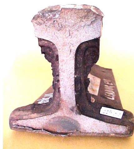
FIG. 51 : 421 - WELDING, THERMIT JOINT TRANSVERSE CRACK
