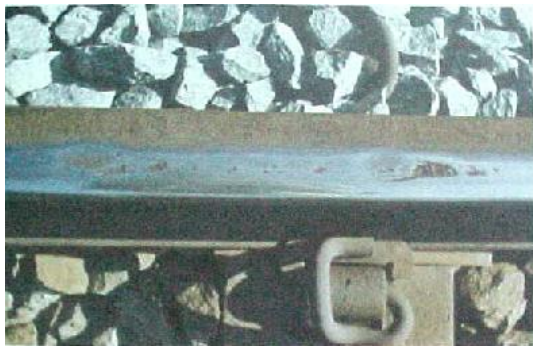
FIG. 40 : 2252 - HEAD SURFACE, WHEEL BURN REPEATED
